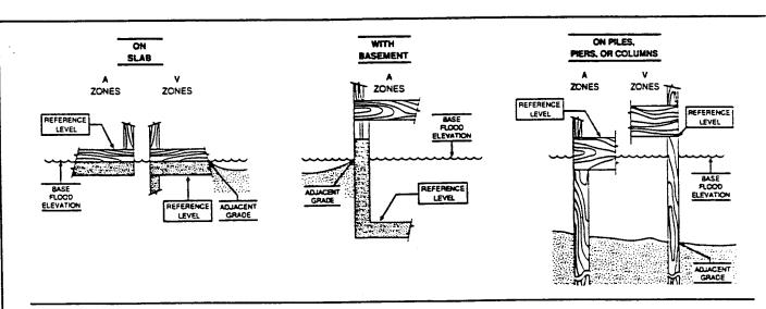
The diagrams above illustrate the points at which the elevations should be measured in A Zones and V Zones.
