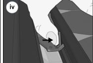
Press down (iii) and then inwards (iv) on the tail of the T-Lock to fully secure the Array Skirt.
