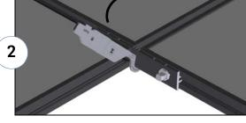
Use the Flat Tool to rotate the Interlock out of the Zep Groove.
