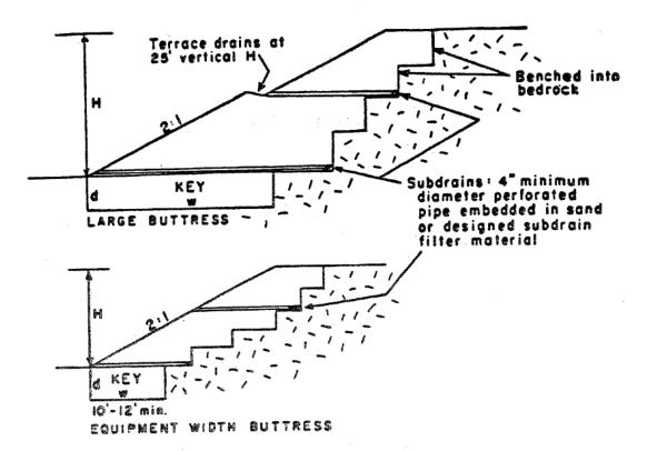
A buttress fill is an engineered support structure design with parameters based upon a slope stability analysis. The key width (w) and depth (d), the buttress heighth (K) and mass are designed by the soil engineer to support a slope that has a potential for failure. Subdrains are necessary and the filter material should be designed by the soil engineer.
