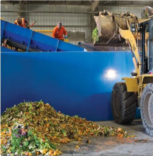
Central Marin Sanitation Agency (CMSA) in San Rafael, California receives commercial food waste collected and preprocessed by Marin Sanitary Service, then taken to CMSA for codigestion. Photo courtesy of Marin Sanitary Service
