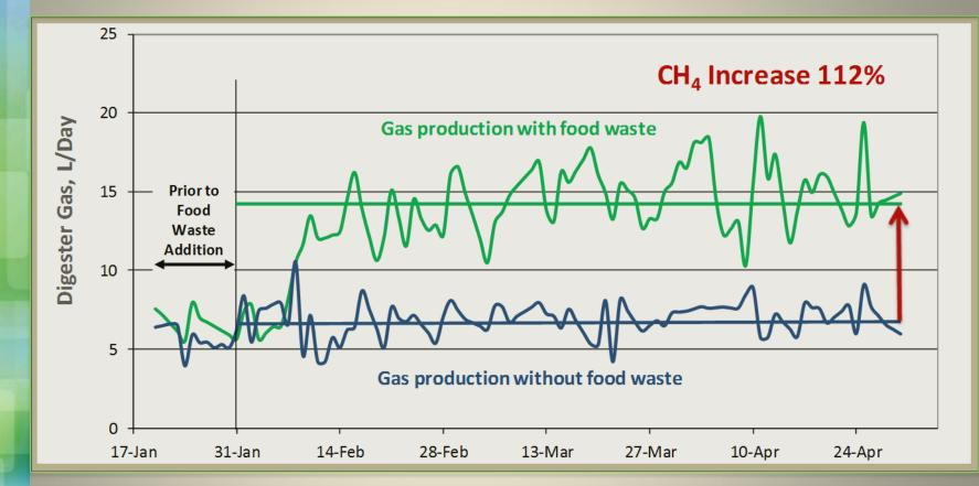
Adding 10-12% (v/v) food waste slurry to sludge could <u>double</u> biogas production
