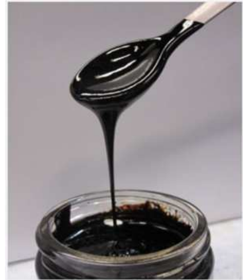
Enlarge / Biocrude oil, produced from wastewater treatment plant sludge, looks and performs virtually like fossil petroleum.
