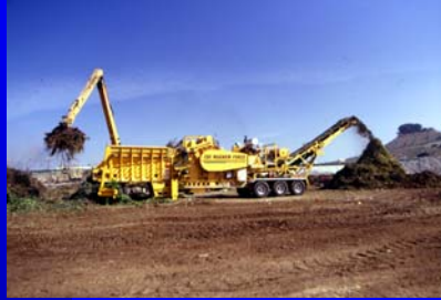
Green waste grinding.
