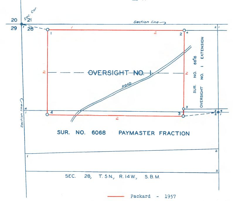
This survey was made with a C. L. Berger & Sons transit No. 28625, with horizontal limb 5 ins. dism., having two double opposite verniers and full vertical circle 5 ins. dism., having one double vernier; the verniers read to one minute of arc. The instrument was in good condition at the time of the survey and all adjustments were in good order.
