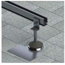
6. Attach the rail to the L-foot using a 3/8" bolt, star washer and nut. Recommended Torque 14 (ft. lbs.).
