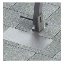
1. Attach the extension bar to the flash L- base using the M8 bolt, nut and star washer. Place star washer between the extention bar and L-foot.
