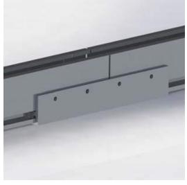
2. Slide the next rail section into the splice. From 1/4" to 1/16" (check with county requirement) between the rail ends. This allows the splice to act as an expansion joint.
