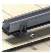
7.Attach the rail to the tile hook using 3/8" bolts and nut. (It's recommended to place a star washer betweenthe r ail and flat tile hook).
