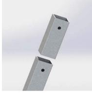
2. If the extension bar is longer then required, cut the extension bar and drill a holes using a  $1/4^{"}$  dril bit  $0.8^{"}$  below the cut line.
