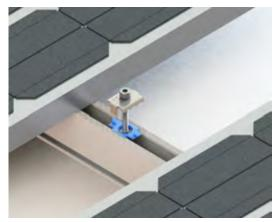
3- Verify that the Channel Strut is locked in the rail channel, using the Channel Strut Floater position (now parallel to rail channel) as a guide. Place the module(s) under the Grounding Mid Clamp, making sure the Grounding Mid Clamp teeth are in line with the module frame.
