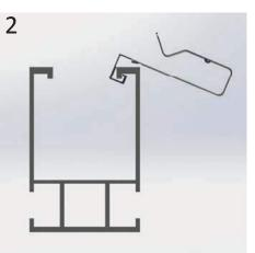
2. Lower the cable clip towards the side of the Dual rail.
