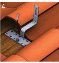
4. Attach the roof hooks to the rafter using the three (3/16") or two (5/16") hex bolts, embedded a minimum 2.5".
