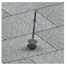
1. Drill a pilot hole using 3/16" drill bit through the roof material and into the center of the rafter at the planned location.
