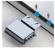
2. Lower or slide the channel strut through the Dual rail gap.
