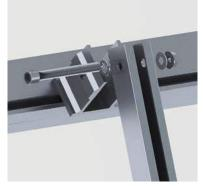
6. Secure the U-bracket to the extension bar using the M8 bolt, nut and star washer. Place star washer between the extension bar and U-Bracket.
