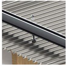
6.Attach the rail to the hanger bolt using the star washer, flat washer and 3/8" bolt.
