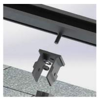
3. Slide the 3/8" bolt through the back side channel of the rail and attach to the upper leg base. Place one star washer between the rail and upper U-bracket
