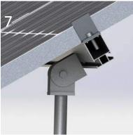
7. For rails on the low end of the module use an angle bracket. Place one star washer between the rail and angle bracket.
