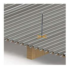
1. Drill a pilot hole using 5/16" drill bit through the roof material and into the center of the rafter at the planned location.
