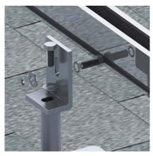
5. Attach the L-foot to the standoff using a 3/8" bolt, star washer and flat washer.
