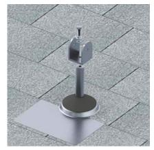
1.Attach the angle bracket to the standoff and secure it using the bolt. Make sure the order of the star washer and the flat washer is as shown a above. Tightening torque (14 ft. lbs).
