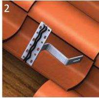
2. Insert the three (3/16") or two (5/16") bolts through the washer and S-Tile hook and apply fresh compatible sealant to the base.
