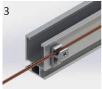
Push the grounding conductor (ground wire to be at minimum 10Ga)all the way to the back of the U shaped slot and tighten the screw to (3 ft. lbs).
