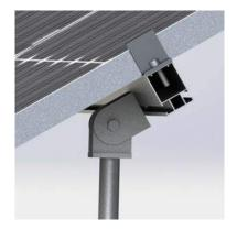
6. For rails on the low end of the module use an angle bracket. Place one star washer between the rail and angle bracket.
