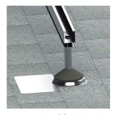
6. Screw the 3/8" bolt to the standoff. Recommended Torque 14 (ft. lbs.)
