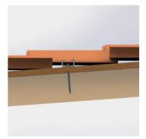
4. Screw the 5/16" lag bolt into rafter, embedded a minimum 2.5". Tightening torque is dependent on the roof material.
