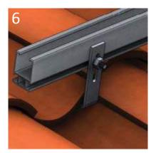
6. Attach the rail to the tile hook using 3/8" bolts and nut. (it's recommended to place the star washer between the rail and S-tile hook.
