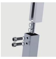
2. If the extension bar is longer than required, lightly loosen the two M8 bolts and slide the adjustable bar up or down as necessary and retighten the two M8 bolts.
