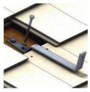
4. Attach the roof hook to the rafter using the two (3/16" or 5/16") hex bolts, embedded a minimum 2.5". Tighening torque is dependent on the roofing material.
