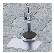
1. Attach the lower extension leg base to the Dual Jack "standoff" using the 3/8" bolt, star washer & flat washer.
