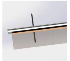
2. Screw the hanger bolt into the rafter, embedded a min. 2.5". Tightening torque is dependent on the roof material.
