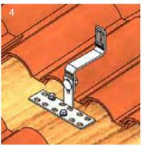
4. Attach the tile hook to the rafter using the three (3/16'') or two (5/16'') lag bolts, embedded a min. of 2.5"
