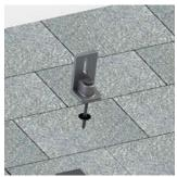
3. Put 5/16" x 5" lag bolt through L-foot. Next, slide the EPDM washer up onto the lag bolt.
