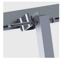
6. Secure the upper leg base to the extension bar using the M8 bolt, nut and star washer. Place one star washer between the U-bracket and extension bar.
