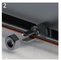
2. Tightening the grounding lug to (7 ft. lbs) make sure the back plate teeth is biting the rail.
