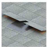
2. Gently break seal between shingles and remove any nails. Slide flashing up under shingles, with flashing lined up with rafter center. (Marked center in step #1.)
