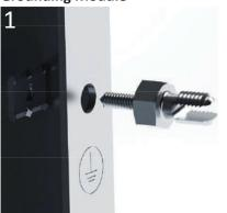
1. Slide the grounding lug through the modules grounding hole and attach to the back plate. Tightening tourg (7 ft. lbs) make sure the back plate teeth is bitting the module frame.
