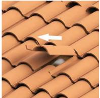
1. Remove the tile and locate the rafter.
