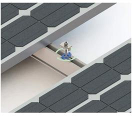
2- Lock the Channel Strut in the Dual Rack Rail channel by turning the Channel Strut Floater 180 degrees, which will ensure the grooves on the Channel Strut will line up with the lip of the Dual Rack Rail channel.
