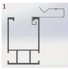
1. Place the cable clip on one of the Dual rail sides making a 90° angle.
