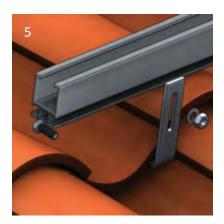
5. Slide the 3/8" T-bolt through the rail groove.
