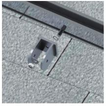
2. Slide the 3/8" bolt though the back side of channel of the rail and attach to the angle bracket. Place one star washer between the rail and angle bracket. (Tightening torque 14 ft.lbs).
