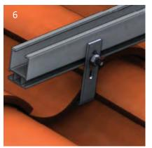
6. Attach the rail to the tile using 3/8" bolts, washer & nut. (Recommended: place star washer between the rail & S-tile adjustable hook).
