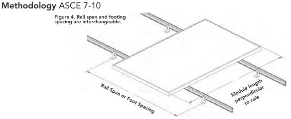
Note: Modules must be centered symmetrically on the rails (+/- 2\*), as shown.
