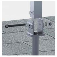
2. Align the extension bar holes with the leg base holes and secure it with the M8 bolt and nut. Place one star washer between U-bracket and extensio n bar.
