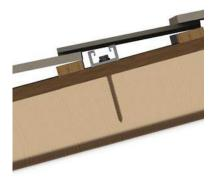
4. Screw the 5/16" lag bolt into rafter, embedded a minimum 2.5". Tightening torque is dependent on the roof material.
