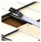
2. Insert the two (3 /16" or 5/16") bolts through EPDM washers and the flat hook and apply fresh compatible sealant to the base.
