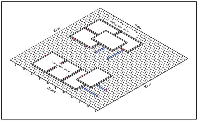
Figure 6. Rails may be placed parallel or perpendicular to rafters.
