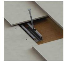
2. & 3. Insert the lag bolt through the tile strut and apply compatible sealant.
