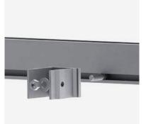
3. Slide the 3/8" bolt through the back side channel of the rail and attach to the U-bracket. Place one star washer between the rail and U-bracket.
