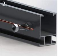
(7ft. lbs) make sure the back plate teeth is biting the rail.
