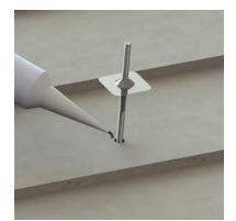
8. Apply fresh compatibale sealant to seal the tile openinig and lower the mini flashing.
