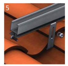
5. Slide the 3/8" bolt through the rail groove.
