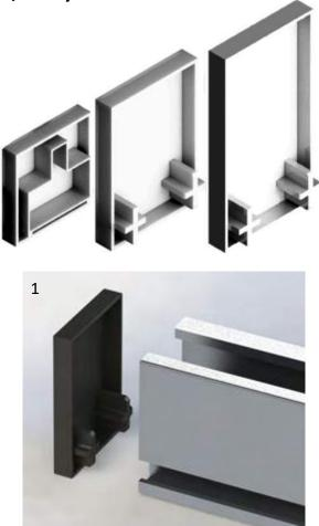
**1.** Align the bottom teeth of the End Cap with the opening rail grooves.
