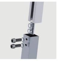
2. If the extension bar is longer than required, slightly loosen the two M8 bolts and slide the adjustable bar up or down as necessary and retighten the two bolts.
