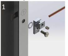
1. Slide the grounding lug through the module's grounding hole and attach to the back plate. (Tightening torque 7 ft. lbs). Make sure the back plate teeth are biting the module frame.
