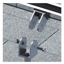
3. Align the angle bracket hole and secure it with the bolt and star washer, as shown above. (Tightening torque 14 ft.lbs).
