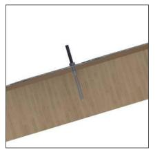
2. Screw the 5/16'' lag bolt into rafter, embedded minimum 2.5''. Tightening torque is dependent on the roofing material.
