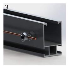
3. Push the grounding conductor (ground wire to be at minimum 10Ga) all the way to the back of the U shape bolt. Add the nut in secure to (2 ft. lbs).
