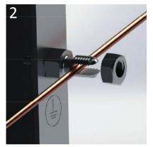
2. Insert the grounding conductor (ground wire to be at minimum 10Ga) and push it all the way to the back of the U shape bolt.
