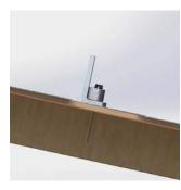
5. Screw the 5/16" lag bolt into the rafter, embedded a minimum 2.5". Tightening torque is dependent on the roofing material.
