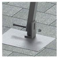
1. Attach the extension bar to the flash L- base using the M8 bolt, nut and star washer. Place one star washer between the extension bar and L-foot.
