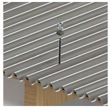
3. Place the EPDM, flat washer and nut and secure the bolt. (Tightening torque dependent on the roof material).
