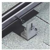
7. Attach the rail to the L-foot using 3/8" bolt, nut and star washer. The Star washer must be placed between the rail and L-Foot.
