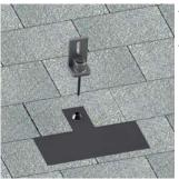
4. Secure EPDM washer onto bolt. Attach bolt and flashing to rooftop.
