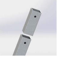
3. If the extension bar is longer than required, cut the extension bar and drill a hole using a 1/4" drill bit 0.8" below the cut line.
