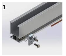
1. Slide the grounding lug through the rail groove.
