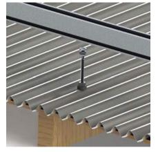
4. Place the second bolt and lower it to the planned rail height above the roof.
