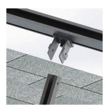
6. Move the rail to align all the upper leg bases with their extension bars.
