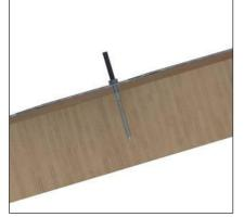
2. Insert the lag bolt through the 1.5" washer and 1.5" EPDM. Screw the 5/16" lag bolt into rafter, embedded min. 2.5".
