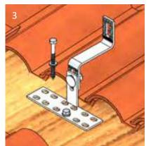
3. Insert the three (3/16") or two (5/16") bolts through the washer and S-tile hook, and apply fresh compatible sealant to the base. Tightening torque is dependent on the roof material. Adjust S-Tile hook height accordingly. Tighten the M8 flange nut.
