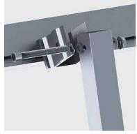
5. Secure the upper leg base to the extension bar using the M8 bolt, nut and star washer. Place star washer between the extension bar and U-bracket.
