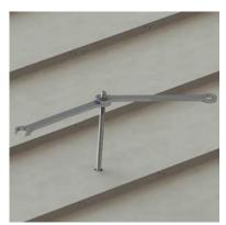
7. Use the two 3/8" nuts to engage the threaded headless bolt to the channel strut below the tile and remove the nut when done.
