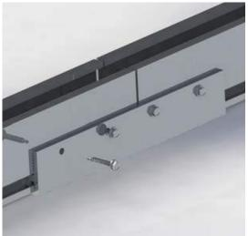
3. Tighten the first self-tapping screw all the way into the rail and tightening the rest until they just contract the rail, leaving it it just loose enough for the rail to expand and contract within the splice. For rigid joint screw all the self tapping screws all the way into the rail. The choice between thermal expansion or rigid joints depends on the installation area.
