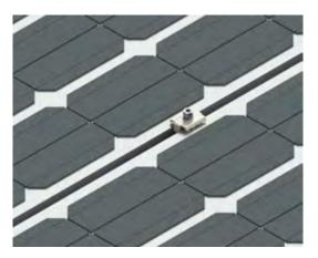
4- Make Sure the Grounding Mid Clamp teeth are "biting" center of the module frames to ensure electrical grounding continuity. Screw the M8 bolt (10 ft.-lb. torque recommended) and the Channel Strut will align itself with the Dual Rack Rail grooves.
