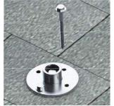
2. & 3. Screw the 5/16" lag bolt into the rafter, embedded minimum 2.5". Tightening torque is dependent on the roofing material.
