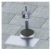
1. Attach the lower extension leg base to the Dual Jack "standoff" using the 3/8" bolt, star washer and flat washer.
