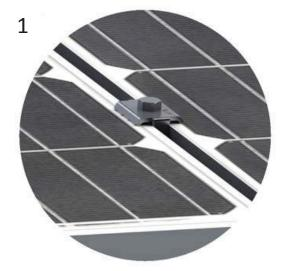
1. Grounding mid clamp electrically bonds the module's frames together. (Up to 44 modules per #6 bare copper wire.)
