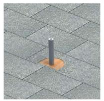
1. After securing the Dual Jack roof attachment to the roof, cut a piece of the shingle if required.
