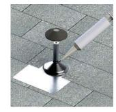
5. & 6. Install the flashing over the standoff and add the EPDM collar. Please refer to page [3.6] for detailed flashing installation.
