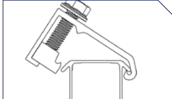
Tilt and hook the mount around the top "dog ear" of the rail
