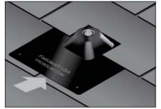
Step 5: Slide FastJack<sup>®</sup> flashing under shingle apply sealant on right and left side of flashing
