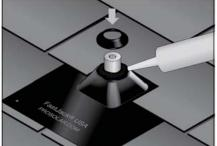
Step 7: Apply 1/4" bead of sealant (Geocel 4500) and compress with aluminum collar
