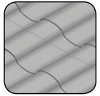
STEP 1: Select a tile in the area of the roof rafter and snap a line down the midsection of the tile.
