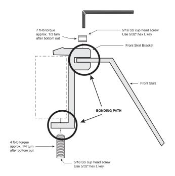
Skirt NOT required for class A sloped roof fire rating. Type 1 and 2 modules.
