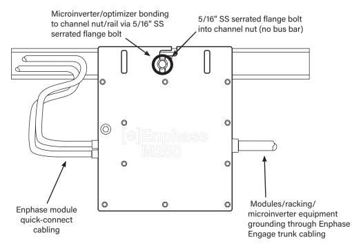
BASIC BONDING/GROUNDING THROUGH ENPHASE ENGAGE CABLE DIAGRAM
