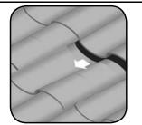
STEP 2: Remove the tile by pushing and pulling. It is usually held in place by a small nail.
