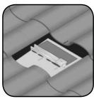
Step 8: After bolting the base to the roof, slide the upper carriage under any portion of the crown (high point) of the tile." For flat tile, slide the upper carriage near the middle of the tile.\*
