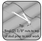
Step 11: Insert threaded stud through tile and hand-tighten to engage with base. Bind two 3/8" nuts (included) using 9/16" wrenches and tighten. and tighten to 15 ft-lbs. Tip: Pre-assemble studs and nuts before roofwork
