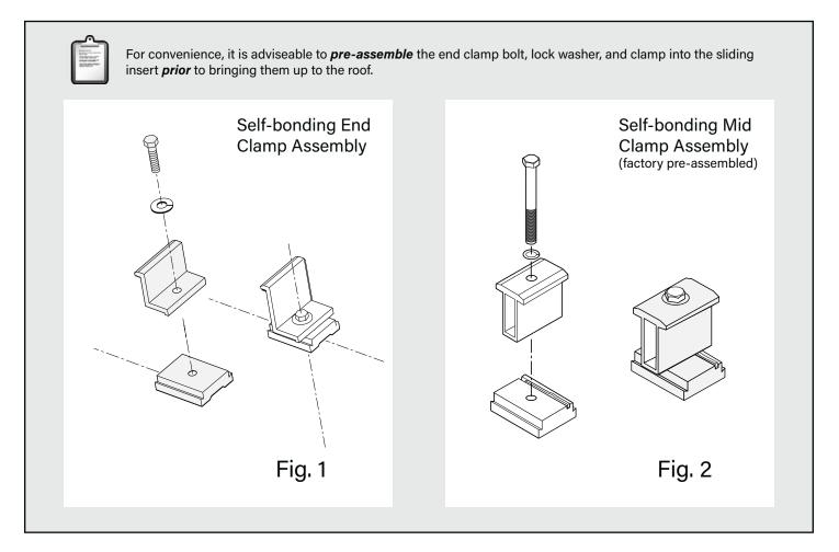
After the support rails have been fastened, you are ready to install the solar modules. There are two sets of clamps: the outside clamps (end clamp) (Fig. 1), and the inter-module clamps (mid clamp) shown (Fig. 2) that install between the modules.
