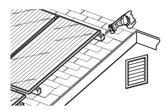
To complete the installation, cut off any excess support rail not being used with a reciprocating saw. Use a file to remove any sharp edges. Per UL2703, it is recommended to periodically re-inspect systems for any loose components or corrosion. Retighten or replace components as necessary.
