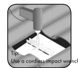
Step 6: Fasten lag screw until seated. Do not overtighten. The sealant should flow outward sealing any holes.
