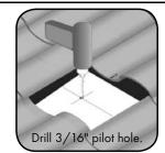
Step 4: Using a 3/16" drill bit, drill pilot hole along the rafter center
