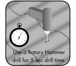
Step 10: Using a 1/2" carbide drill bit and ROTARY HAMMER DRILL in hammer mode, drill through the tile. See online video at www.prosolar.com for details.
