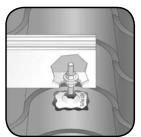
Step 13: Fasten rail with lower and upper 3/8" nuts/washers to 15 ft-lb as shown.
