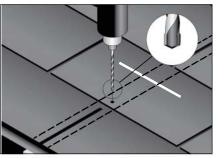
Step 2: Drill rafter pilot hole with 3/16" carbide bit
