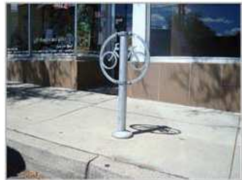
Bicycle parking can also be on a single post to minimize sidewalk obstructions.
