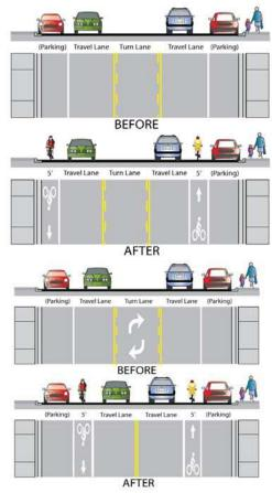
Bike Lanes Will Not Fit – In this last case, the existing roadway geometry will not allow for the addition of bike lanes. Either a bike route or major reconstruction of the roadway may be necessary for bikeway continuity.
