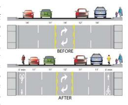
V The County will consider reduced travel lane widths of 10 feet on a case by case basis and as recommended using engineering judgment considering such factors as vehicle speeds, and truck and bus volumes.
