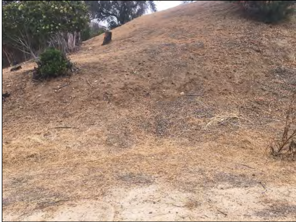
Figure 12. Graded area mapped as Pacoima Formation (Qp), showing Quaternary alluvium (Qa) in the lower flat area (bottom of photo) and partially exposed Qp sediments along the hillside (center of photo). View north.
