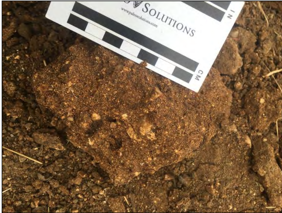
Figure 20. A clasts of Pacoima Formation (Qp) comprising moderately lithified and moderately sorted siltstone and medium grained sandstone with subangular to subrounded plutonic granule to pebble sized clasts. View down.
