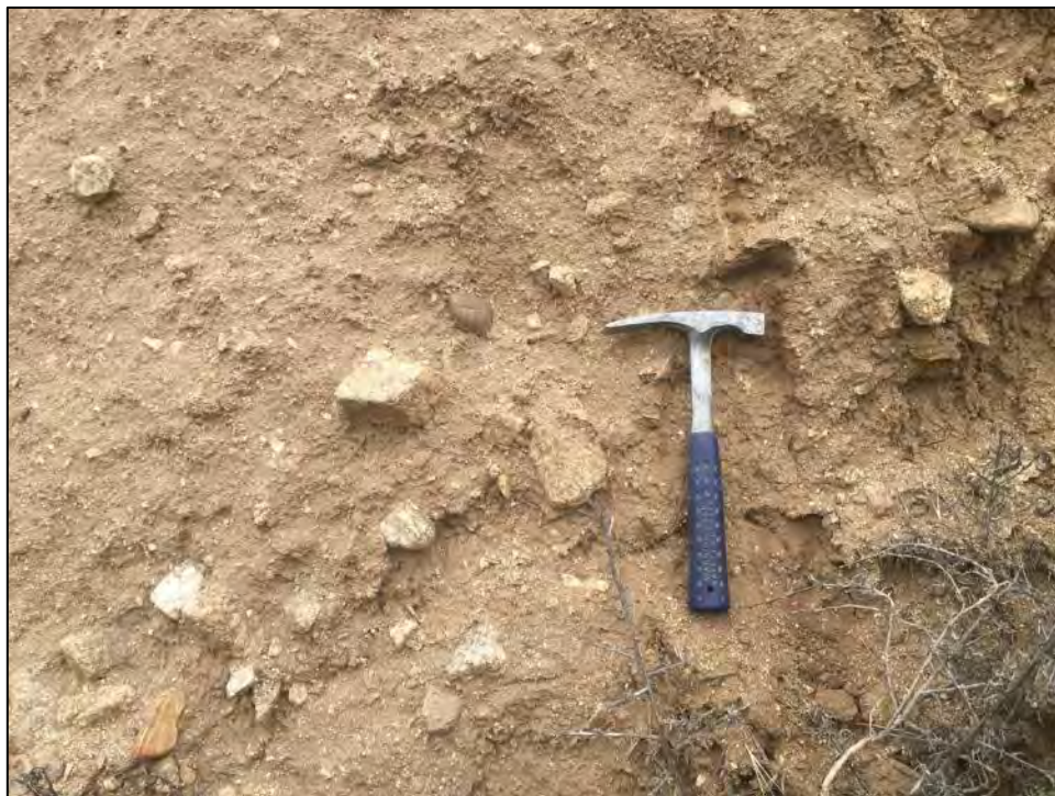
Figure 21. Exposed Pacoima Formation (Qp) sediments comprising massive poorly sorted silt to medium sandstone with subangular to subrounded plutonic pebble to cobble sized clasts. View west.
