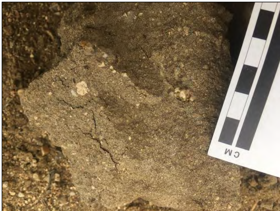
Figure 19. A clasts of Pacoima Formation (Qp) comprising moderately lithified and moderately sorted siltstone and medium grained sandstone with subangular to subrounded plutonic granule to pebble sized clasts. View down.
