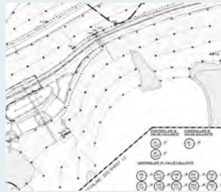
TEMPORARY (2-3 YEARS) ON-GRADE IRRIGATION SYSTEM "OVERHEAD ROTOR SPRAY" (FOR LARGER HYDROSEEDED AREAS)
