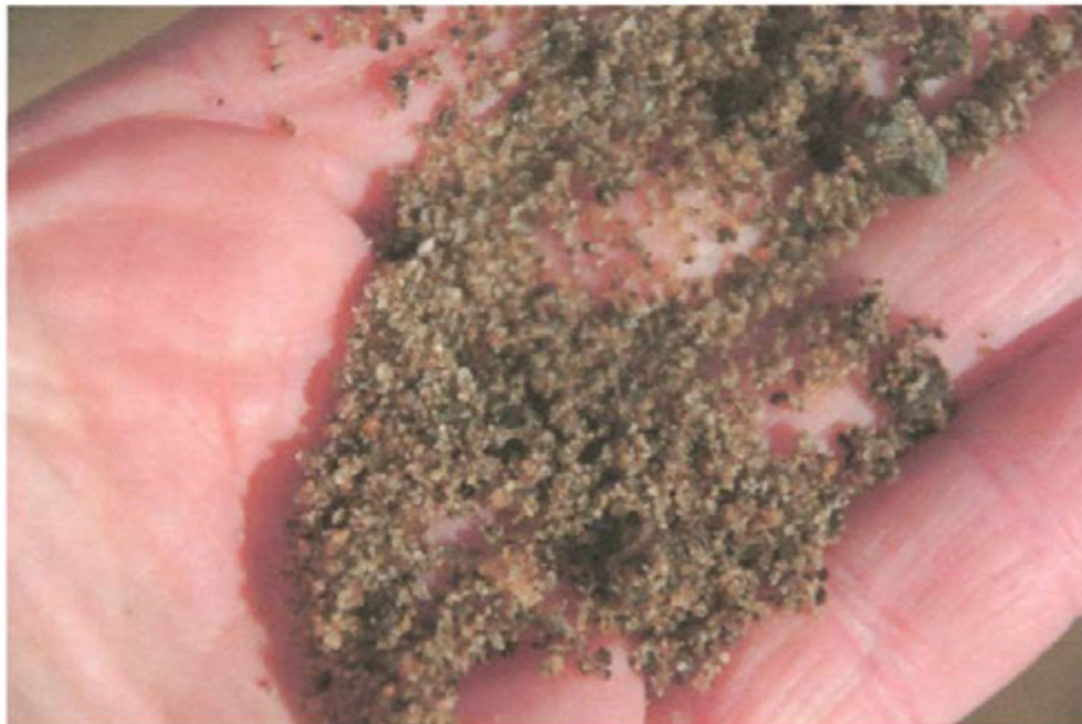
Photo 6: Coarse Sand Observed in Sediments in Terminal Basin
