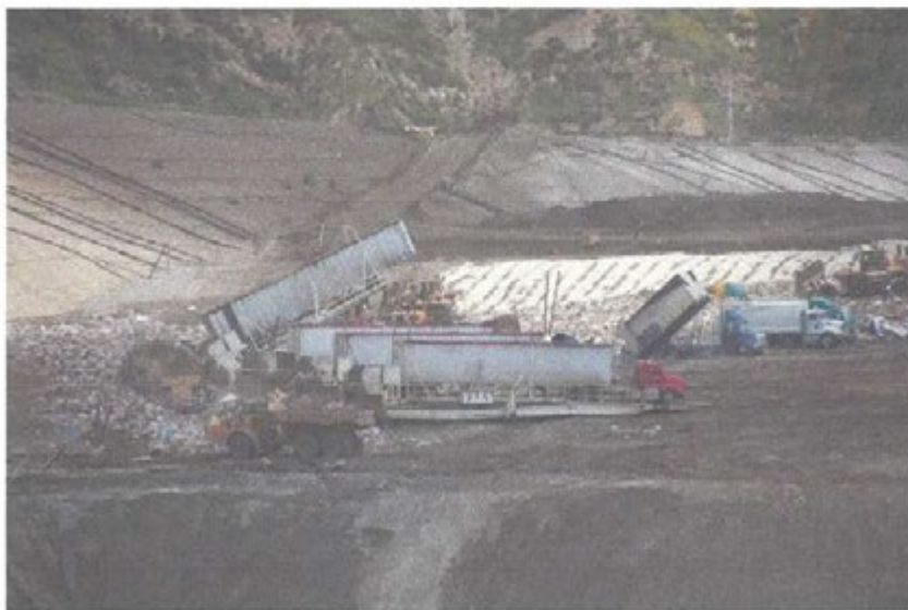
Photo 2: Four tilters in use for waste placement at Cell CC4
