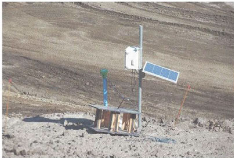
Figure 18: additional monitoring instrument on slope of excavated area of future buttress
