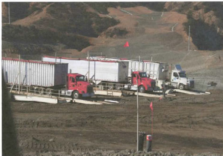
Photo 3: Tilters in use at waste face on Cell CC4 Part 1
