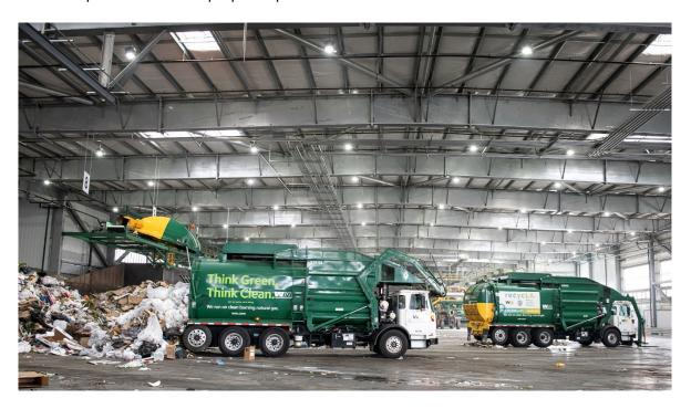
The transfer station is permitted for 4,000 tpd of municipal solid waste (MSW) transfer. Public and private waste collection trucks, typically with 40-yard capacity, drop off MSW. The MSW is consolidated and loaded into transfer trailer trucks that transport the MSW to landfills in or near Los Angeles for proper disposal.
