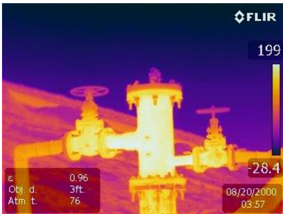
Photo 6. FLIR image of gas well with temperature range up to 199°F at CCL, November 2, 2023
