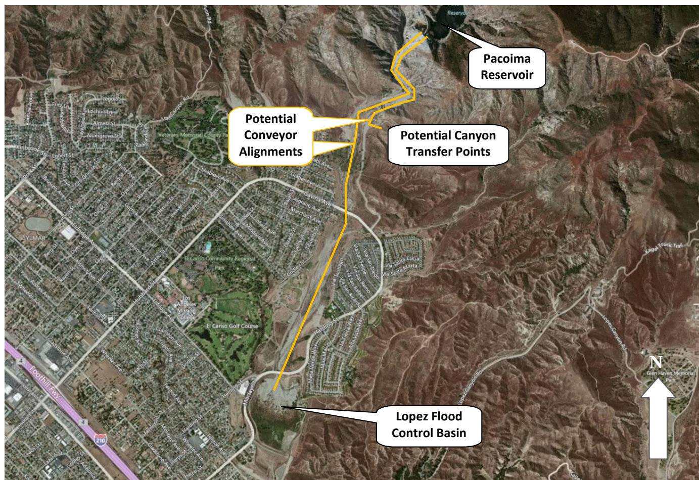
Figure 8-41 Potential conveyor belt alignments
