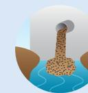
Sluicing involves draining a reservoir to expose the accumulated sediment to incoming water flows so that the water can resuspend the sediment and carry it through the dam's sluice gate or valves. Typically, the sediment-laden water is impounded in a reservoir or other facility downstream that is more accessible for sediment removal operations than the reservoir from which sediment was sluiced. This section focuses on the impacts sluicing has on the reservoir.
