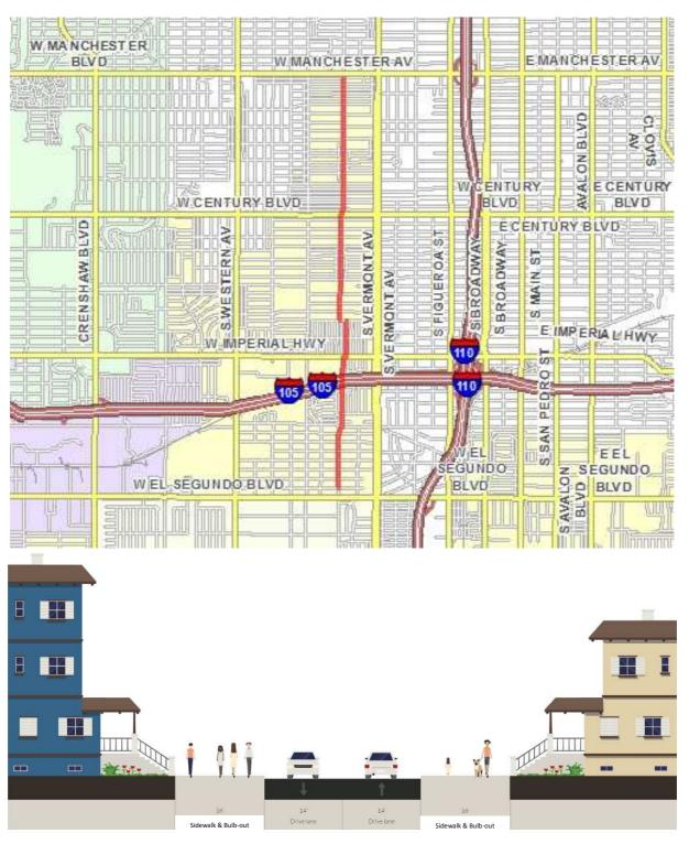
Bulb-outs provide a landing for pedestrians and reduce the crossing distance at the corners.
