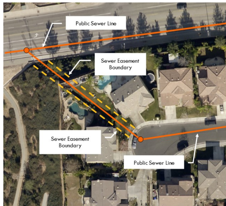
Figure 1: Example of a sewer easement
