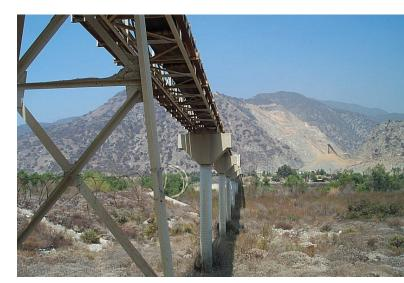
Figure 2-26. Aggregate is carried on a conveyor belt to a processing plant.
