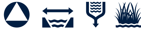
Figure 62. When a symbol is needed that is not available from MUTCD, another symbol in a similar style and weight to MUTCD standards should be used. Examples include of symbols for gender-neutral restrooms, river crossings, a river confluence, and wetlands. Source: (Left) Title 24 of the California Code of Regulations, California Building Code, 2016; all other symbols, River LA.
