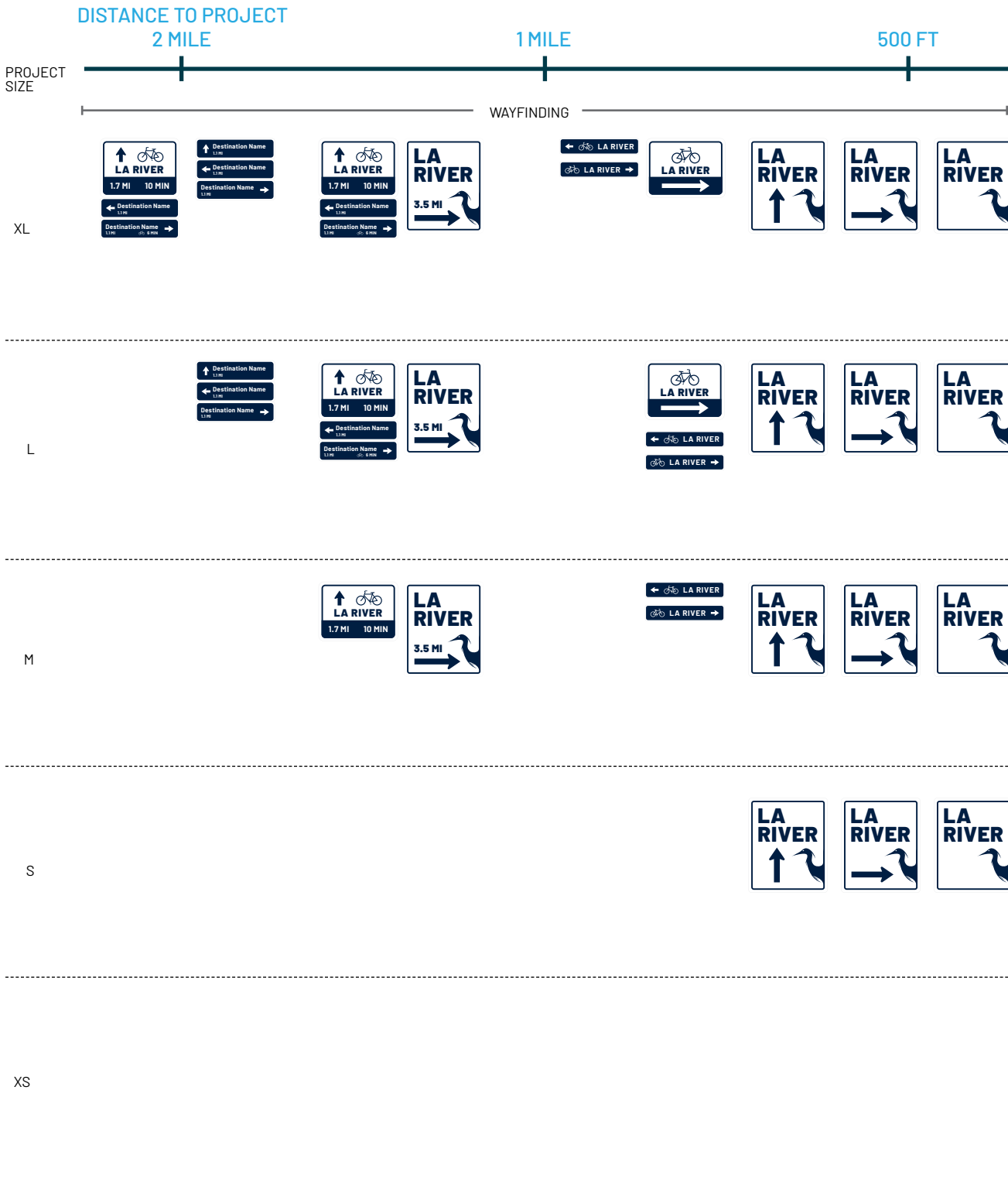
Figure 73. Baseline requirements for environmental graphics leading to the LA River and projects within the LA County Flood Control District right-of-way depend on the scale of the project. Directional signage is required to be two miles away from an XL project, while only required to be 500 feet away from an S project. Directional signage for bicycles are required only for XL-M projects. At gateways, Information signage and Regulatory environmental graphics are required for S-XL projects. Within an XS project, Interpretive, River Mile Pavement Markings, and River Mile Markers are required. Confirmation signs are required with S-XL projects. Incorporation of Large Scale Graphics with L and XL projects should be considered.
