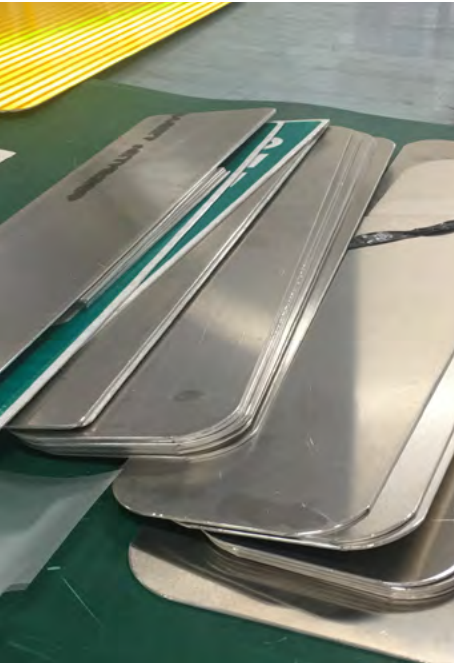
Figure 118. Aluminum with rounded corners is used as the base of many types of signs. Source: OLIN, 2019.
