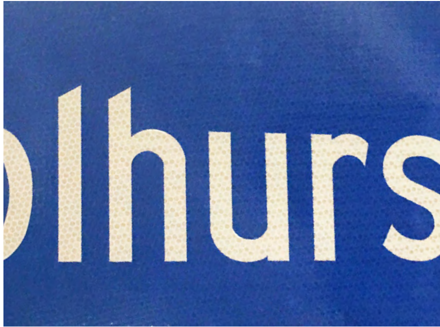
Figure 119. Retroreflective substrates, colored film, and clear anti-graffiti film layer on top of aluminum to create the graphic of a sign. Source: OLIN, 2019.
