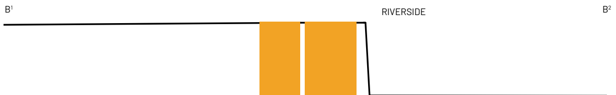
Figure 36. Trails may be consolidated when a wide landside ROW is present. When the trails are consolidated, more land becomes available for parks, planting, and habitat. This figure represents one possible configuration of this typology.
