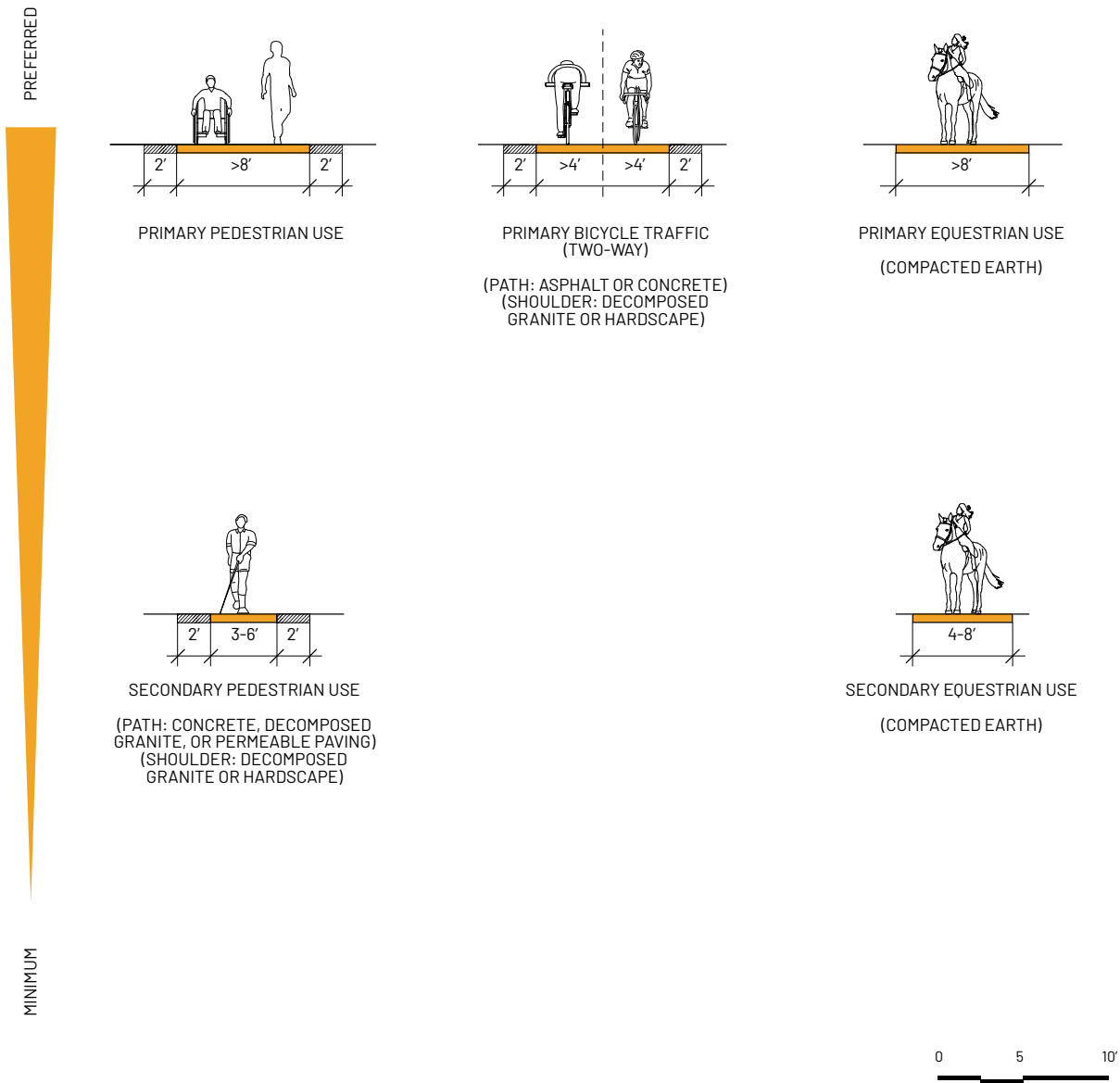
Figure 33. Pedestrian, bicycle, and equestrian trail components vary in width and are most often used in combination with one another, but they may also be implemented as standalone trails in certain projects. Dimensions illustrated for bikes are based on the County of LA Bike Plan.
