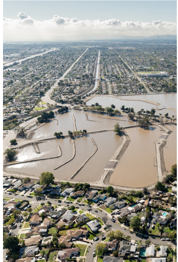
Large spreading grounds, like this one in Pacoima, significantly contribute to the region's local water supply. Source: LA County Public Works, 2018.
